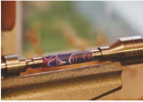
▲ Pic.7 Get close to the bushings, leaving enough to take a fine finishing cut and sanding
